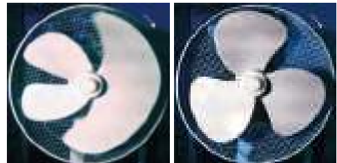
Rolling / Global Shutter: Shot of a rotating fan with different shutter technology.
